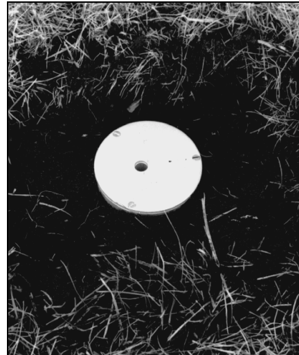
Figure 3-5 Fill In and Pack the Material around the Standard Transducer.
