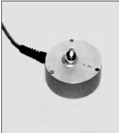
Figure 3-6 Bolting the Standard Transducer to a Surface.
